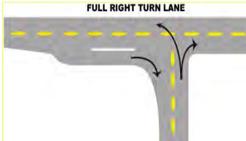
As with any auxiliary turning lane, dedicated right-turn lanes should be designed based on the results of a traffic study.
