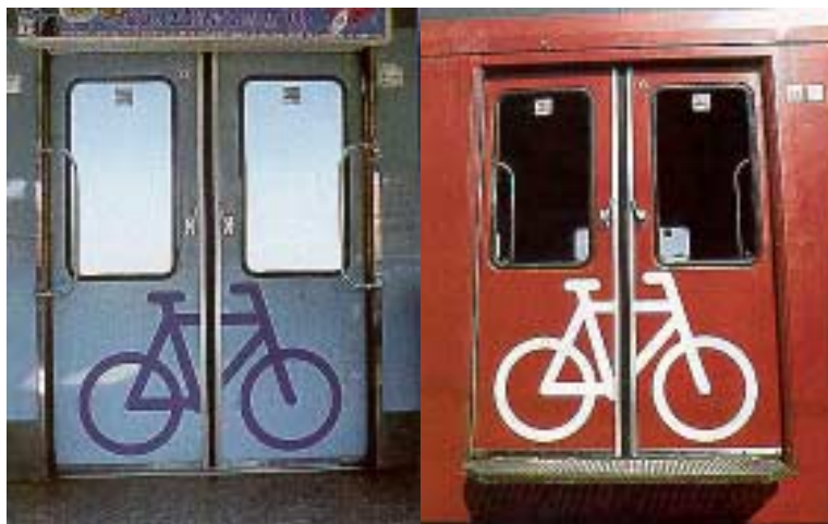
Bicycle stencils on outside and inside doors of Danish State Railways, local "S-Tog" trains indicate those doors where bikes may be brought on board the train.
