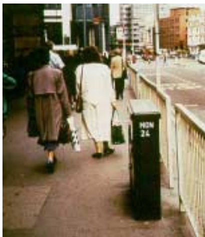
FIGURE 23-6. Pedestrian barriers (separators) are used extensively in London to channel pedestrians to preferred crossing locations.
