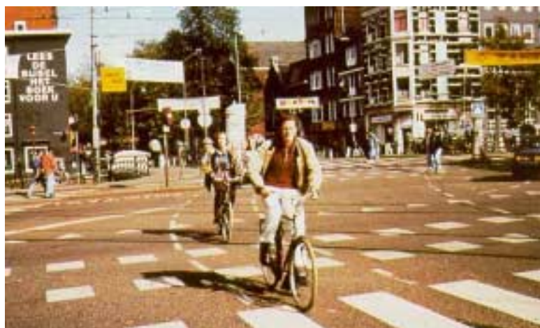
Figure 23-10. Bike lanes are sometimes marked through intersections.
