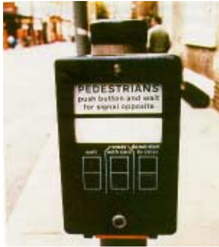
Figure 23-2. Pedestrian push-button hardware in Great Britain gives feedback regarding when to cross.
