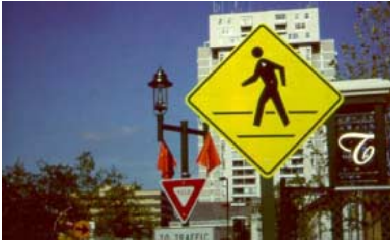
This pedestrian warning sign is fluorescent yellow green (FYG) allowing it to be more visible.
