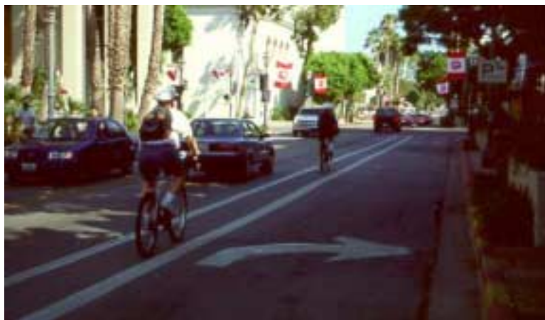
As a temporary solution, striping narrow lanes through intersections may be an option where space is limited.
