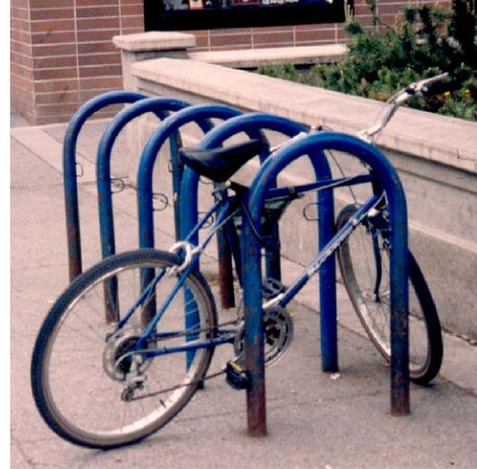
*Bike racks should be in highly visible locations near buildings' main entrances. Select racks that support the bike frame and allow both frame and wheel to be locked.*
