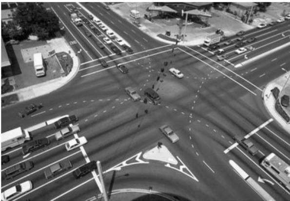
Channelization islands are also used in support of left-turn lanes, forming the ends of the taper approaching the turn bay, and often the narrow divisional island extending to the intersection. At "T"-type intersections, a channelization island can guide oncoming traffic to the right of the left-turn lane.
