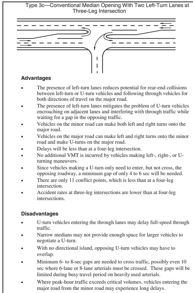
Figure 27. Advantages and disadvantages of median opening type 3c—conventional median opening with two left-turn lanes at three-leg intersection.
