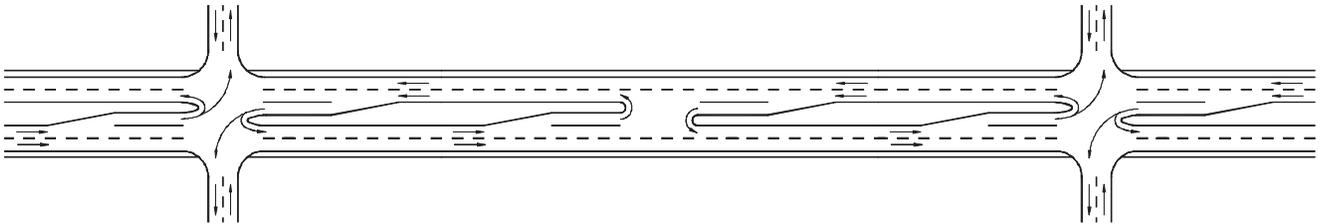
Figure 39. Combination C2—Conventional midblock median opening between four-leg intersections with conventional median openings.
