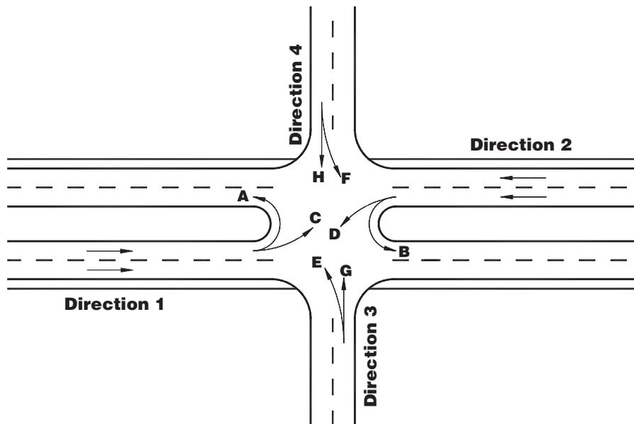
Figure C-20. Turning movements at a four-leg intersection.
