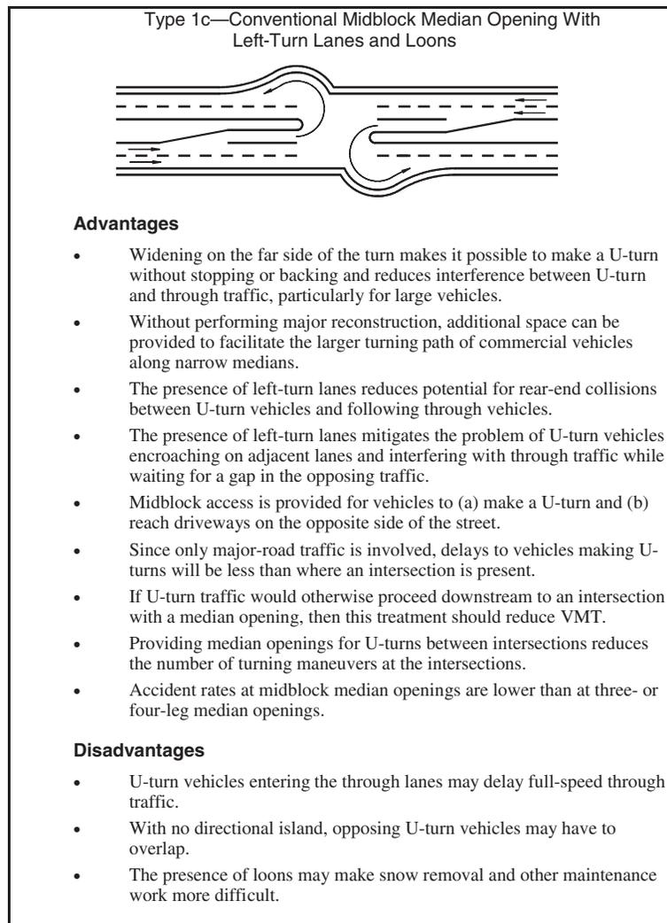
*Figure 21. Advantages and disadvantages of median opening type 1c—conventional midblock median opening with left-turn lanes and loons.*
