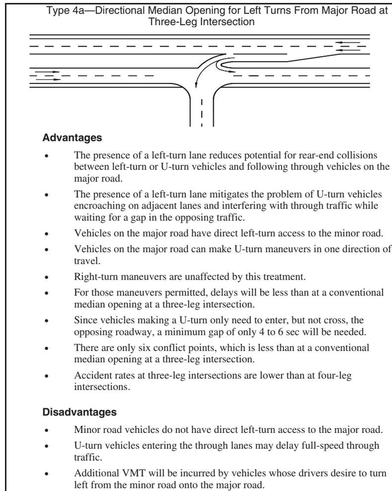
Figure C-13. Advantages and disadvantages of median opening type 4a—directional median opening for left turns from major road at three-leg intersection.
