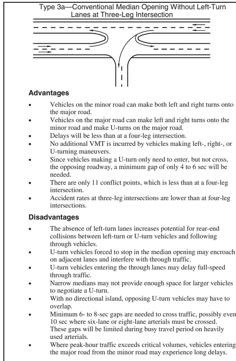
*Figure 25. Advantages and disadvantages of median opening type 3a—conventional median opening without left-turn lanes at three-leg intersection.*
